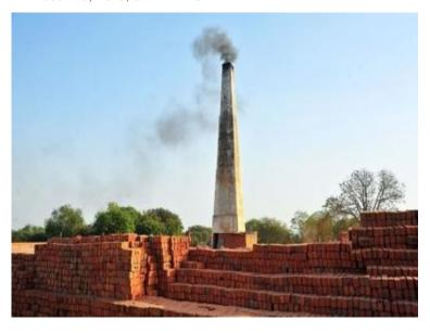
GURGAON: In a first in the city, a brick kiln in Hariyaheda village has started operations after successfully installing the zig-zag technology, which reduces suspended particulate matter and black carbon emissions while saving coal consumption.
